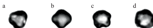
Figure 4: Spherical (a and b) and non-spherical (c and d) coated microbubble oscillation patterns recorded by a ultra high frame rate camera. The forcing frequency was 1.7 MHz for bubbles between 1.5 and 5\mu m , adapted from [5]
