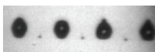
Figure 5: Localized oscillation mode for a microbubble recorded by a ultra high frame rate camera [4]
