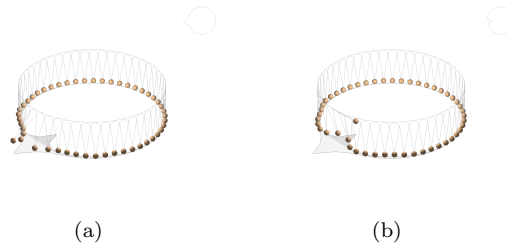
Figure 12: Numerical results of a localized mode (breather) for an excitation of f = 3.04 Hz
