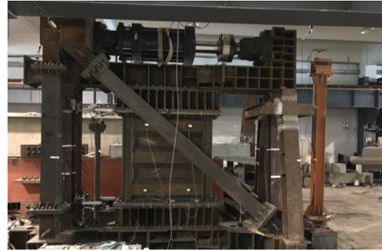
Fig. 15. Self-balanced loading setup
