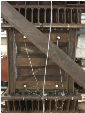
Fig. 21. Buckling of S3 at drift ratio of 1/75
