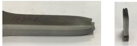
(a) Specimen fracture (b) Separated layer
