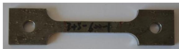
Fig. 5. Photo of one specimen for tests at elevated temperature.
