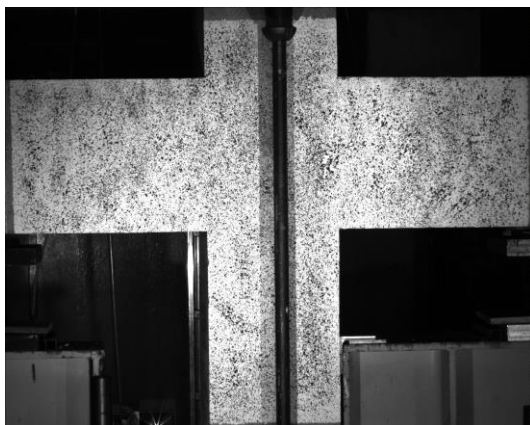
Fig. 7. Surface surveyed by the DIC system.
