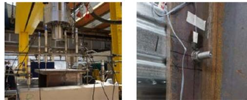
Fig. 5. LVDTs and Strain gauges.
