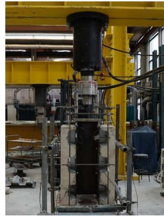
Fig. 4. Push-off test setup.
