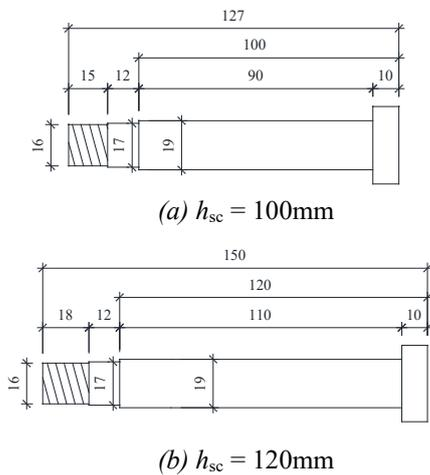
Fig. 1. Dimensions of machined studs.
