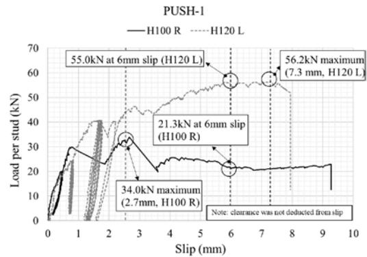
Fig. 6. Comparison of load vs. slip curves (PUSH-1).
