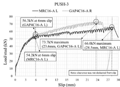
Fig. 10. Comparison of load vs. slip curves (PUSH-3).
