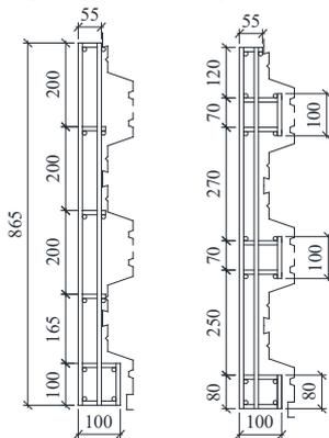
Fig. 3. Design of reinforcement cages (side view).
