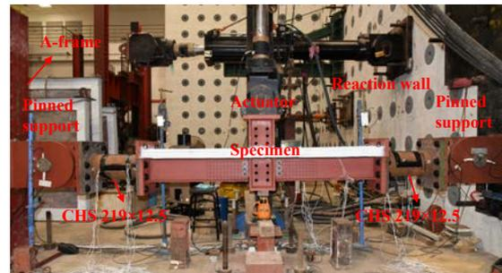
Fig. 1. Front view of quasi-static test set-up.
