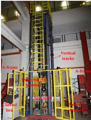
Fig. 2. Front view of impact test set-up.
