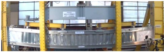
Fig. 13. CWB-SW1 beam – global deformation during the testing.
