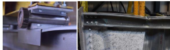
Fig. 18. Local deformations under the load application point.
