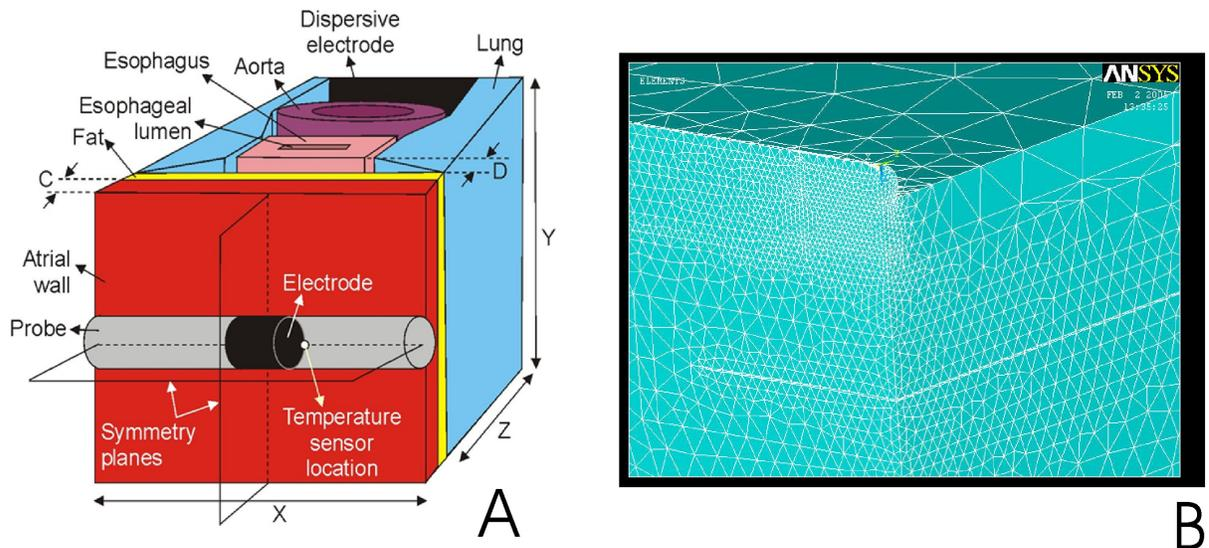
Figure 6.9: A: Theoretical model to study temperature distributions in the esophagus during RF cardiac ablation. B: Detail of the meshing near the electrode.
