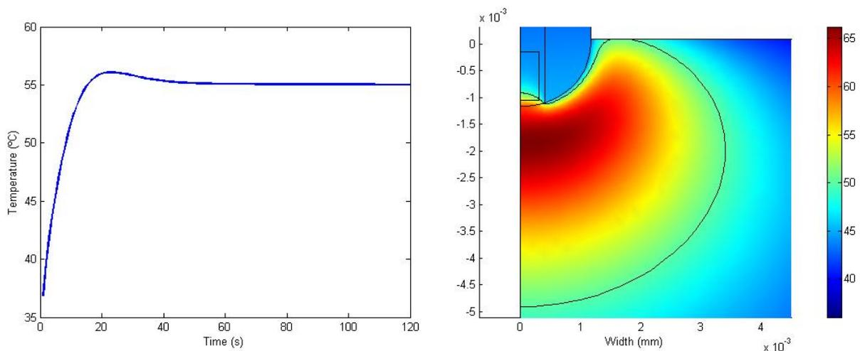
Figure 6.7: Right: Temperature is kept constant at the electrode by modulating the voltage applied. Left: The hottest point is not on the electrode surface but 1 – 2 mm away.
