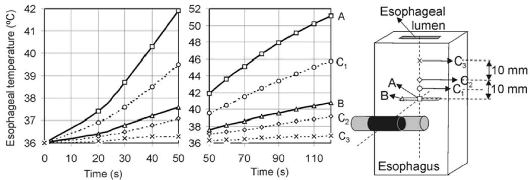
Figure 6.12: Left: temperature evolution at different locations inside the esophagus. Right: Model geometry and nomenclature of the locations.
