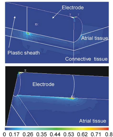
Figure 6.10: Since almost 100% of the electrical power was deposited within 1 mm of the electrode, this suggested that thermal lesions in the esophagus were due exclusively to thermal conduction and not to the deposited electrical power (units in  $10^9 \text{ W/m}^3$ ).
