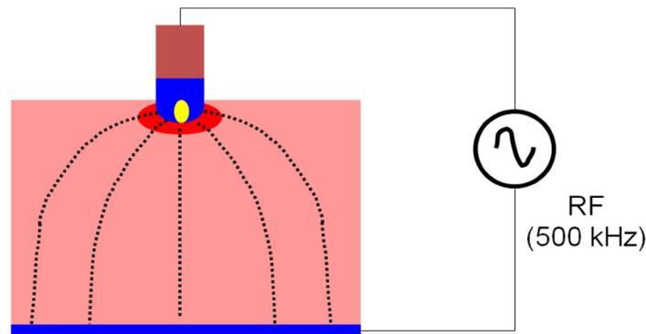
Figure 6.6: Model representing the RF cardiac ablation process.
