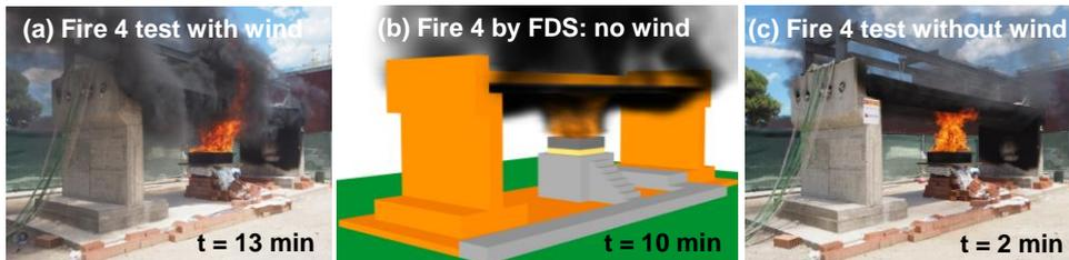
*Figura 7-4. Wind effect in Fire 4: (a) Test 8 with wind, (b) Fire simulation without wind and (c) Test 8 without wind.*
