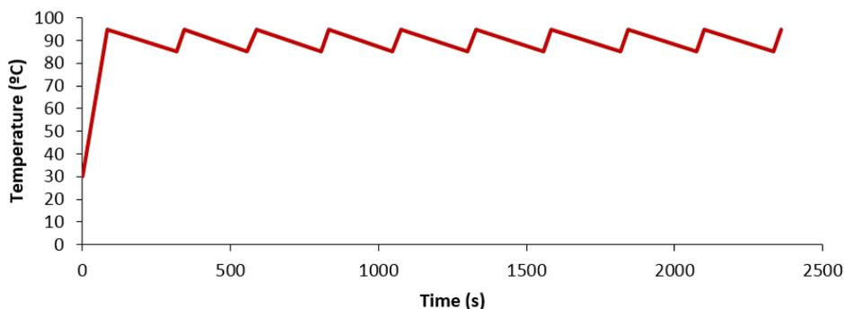
**Fig. 2. Temperature variation of the surface of a 300 W prototype<sup>[26]</sup>.**
