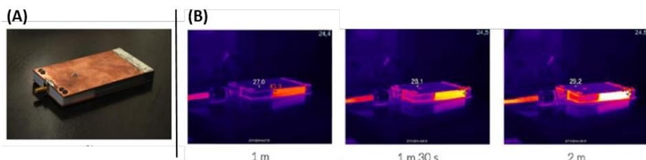
**Fig. 1. Picture of stripline radiators (A) and, (Bb) Thermographies of a heating cycle, applying 30 W microwave power at 2.45 GHz per cell, on the right<sup>[24]</sup>.**
