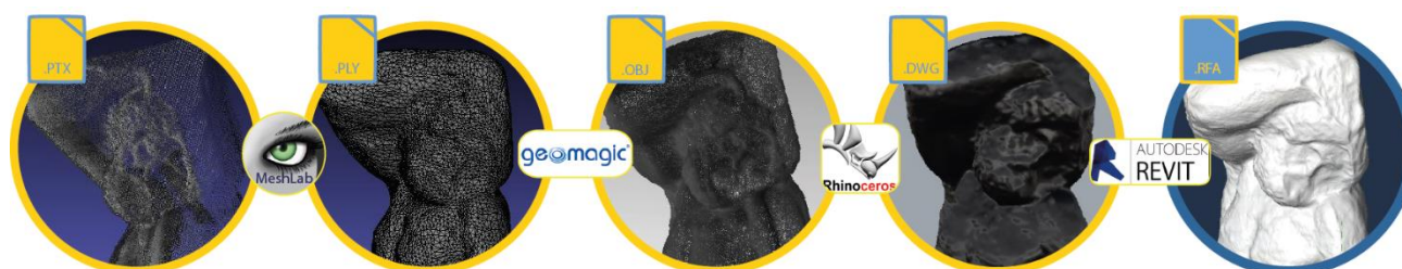
Figure 4: Artwork BIM objects workflow, files and file formats.
