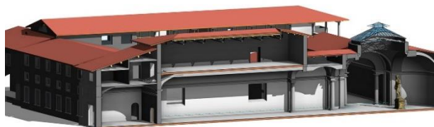
Figure 3: Cross section of the Building Information Model.
