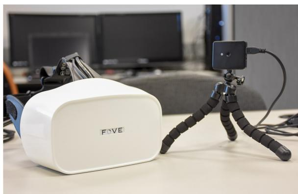
Figure 3.1: FOVE HMD and its head-tracking camera.
