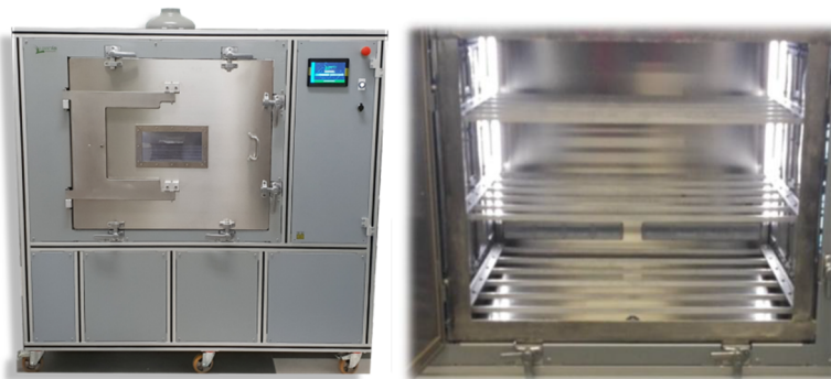
Fig. 2. Front view of the Microwave Processor and internal view of its chamber
