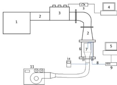
**Figure 1** Microwave fluidized-bed system for drying and disinfection of particles, 1- magnetron, 2- waveguide, 3- three-stub tuner, 4- absorbed power monitoring, 5- data acquisition system and microwave power control, 6- microwave cavity, 7- sample holder (fluidized bed), 8- fibre optic probes, 9- temperature monitor, 10- vents, 11- air blower and heater, 12- air speed potentiometer, 13- air temperature potentiometer, 14- inlet air temperature monitor
