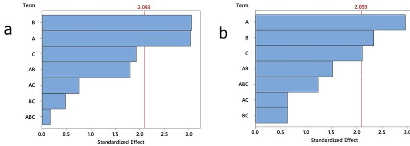
**Figure 6** Pareto Chart of the standardized effects for (a) germination percentage and (b) infected seeds percentage counted after 4d of lentil seeds at 18.5% MC; A = microwave power (0, 300, 400 W), B = air set temperature (50, 60 °C), C = exposure time (5, 10 min);  $\alpha = 0.05$
