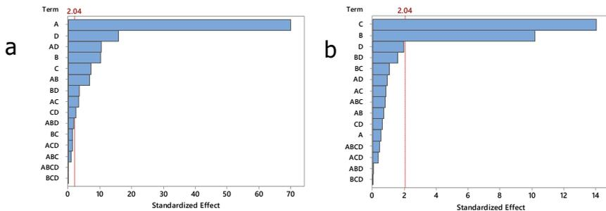
**Figure 4** Pareto Chart of the standardized effects for (a) moisture loss and (b) bed temperature with  $\alpha = 0.05$ ; A = moisture content (10.5%, 18.5%), B = microwave power (0, 300, 400W for 18.5% MC and 0, 400, 500W for 10.5% MC), C = air temperature (50, 60°C), D = exposure time (5, 10 min)
