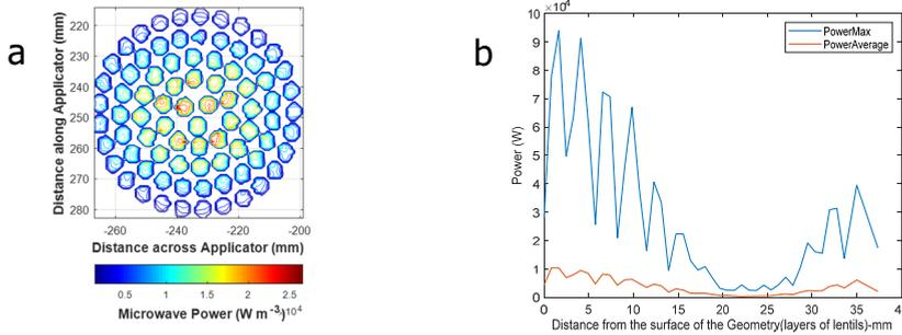
**Figure 2** Power dissipation in lentil seeds, the result of simulation; (a) absorbed power distribution in a cross section of the bottom layer of lentil seeds; (b) vertical maximum and average power density in 100g of lentil seeds in a cylindrical sample holder ( $W/m^3$ )
