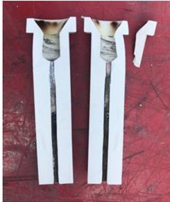
Fig. 5. Thermal shock damage of the AlN tube
