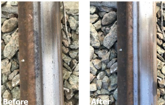
**Fig. 13.** Effect on railhead oxidation
