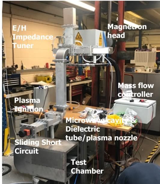
Fig. 3. Laboratory set-up
