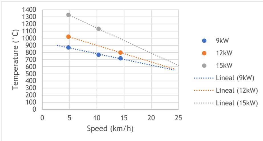
**Fig. 14.** Microwave power/peak temperature vs. Speed dependence, dielectric tube 3 mm
