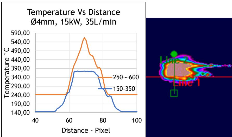
Fig. 10. Thermal images of the rail surface
