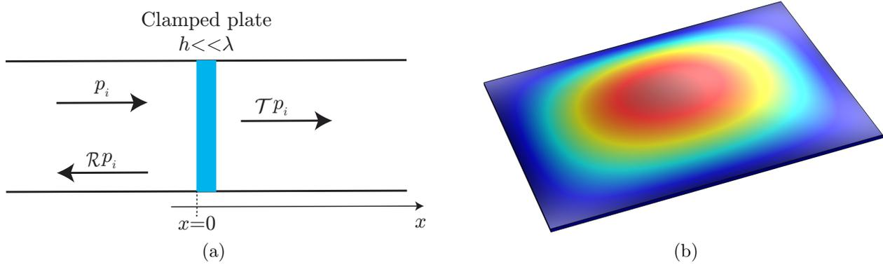
Figure 2: (a) 1-D scheme of the problem in transmission. (b) First mode (piston mode) of the plate.
