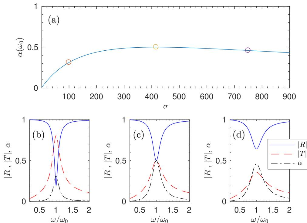
Figure 6: Analysis of the scattering parameters on the losses of the system. (a) represents the absorption of the system at the resonance frequency of the system as the losses increases. Dots in (a) represents the analyzed cases in (b), (c) and (d). (b), (c) and (d) show the scattering coefficients for three particular values of the losses:  $\sigma = 100 \text{ s}^{-1}$ ,  $\sigma = 416 \text{ s}^{-1}$ ,  $\sigma = 750 \text{ s}^{-1}$  respectively.
