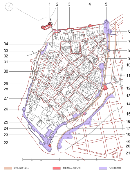
Fig. 2. Chalcis. Kastro. Plan of the fortifications with an indication of the several positions of defense (Modern city's urban tissue in red).
