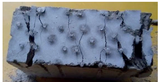
Figure 7: Image of LCTM failure (fiber diameter=1.5 mm).
