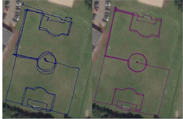
**Figure 4:** Dual-frequency test at the European Space Technology Centre (ESTEC). Samsung S8 (left), Xiaomi Mi-8 (right). Source ESA.
