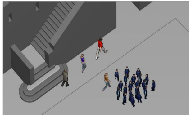
Figure 14: Risk assessment Virtual Tour. Central courtyard. Example of human-human-building interactions in Agent-based simulation (ABM) with BIM.
