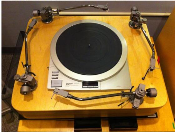
*Turntable used for 78rpm digitization of four simultaneous recordings with different needles.*
