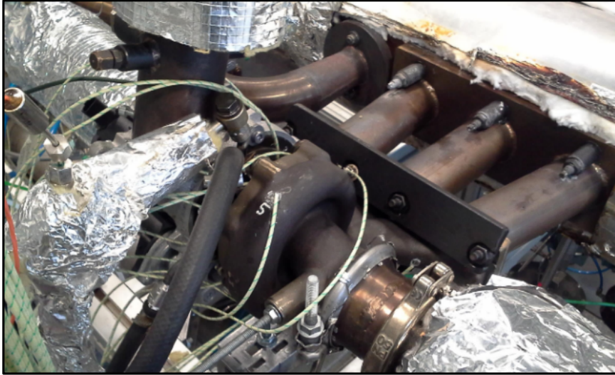
Figure 3.23: Gas stand under thermally exposed configuration for turbocharger testing
