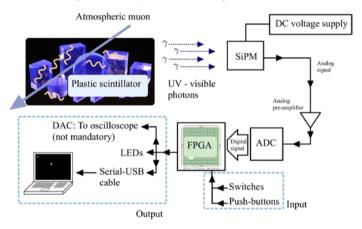
Figure 3. Block diagram of the proposed muon detector showing the roles played by the scintillator, the SiPM, the FPGA, and all the I/O devices integrated on the FPGA development board
