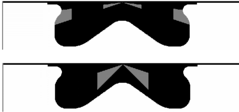
Figure 10 Injection Characteristics with Computational Transfer. 156° Spray Angle (top) and 120° (bottom)
