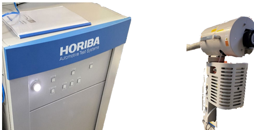
Figure 2: HORIBA HyEVO prototype hydrogen exhaust analyser
