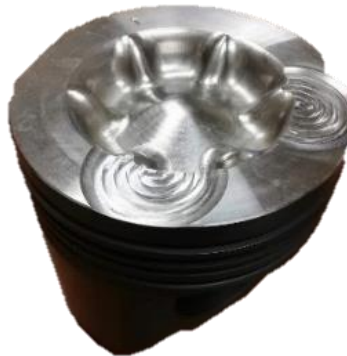
Fig. 3. High compression ratio (CR = 22:1) wave piston
