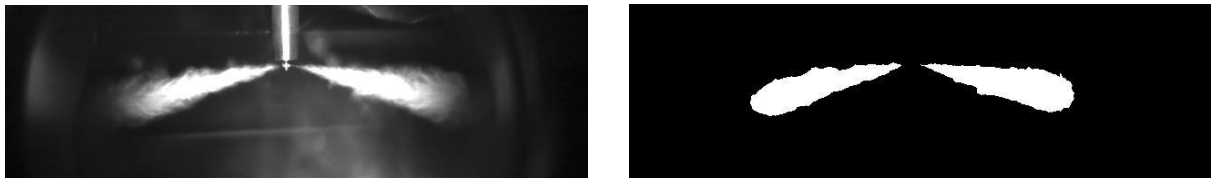
Figure 9 Diesel Spray (Video Sequence) of a 2-Hole Injector (left) and the Binary File (right)
