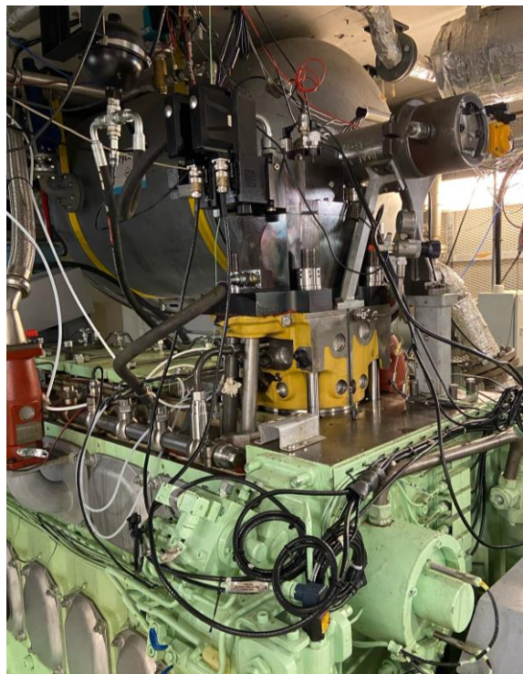
Figure 1 Wärtsilä W20DF research engine in single-cylinder configuration.
