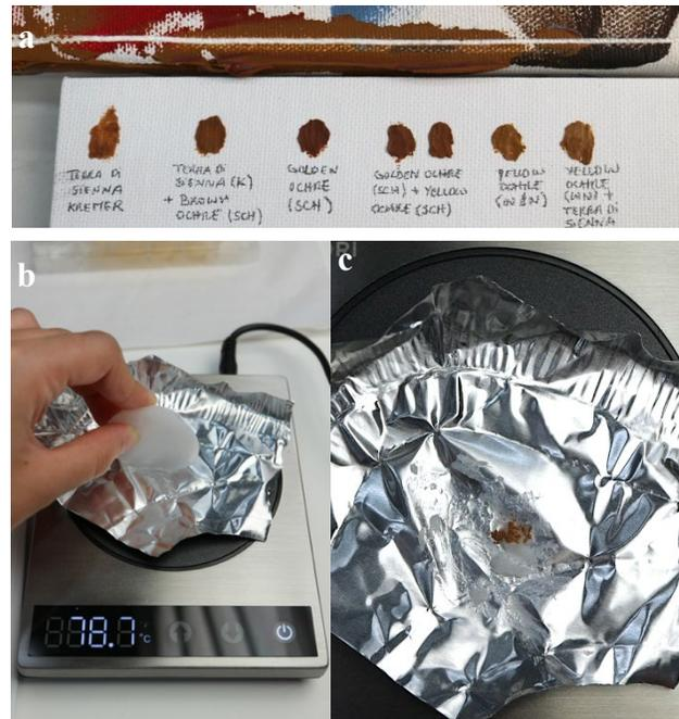
**Figure 9** – a) Colour matching evaluation of fills with different pigments; b) WR mixture being melted on a small hot plate (coffee mug warmer); c) pigments added to the WR mixture while on the hot plate
