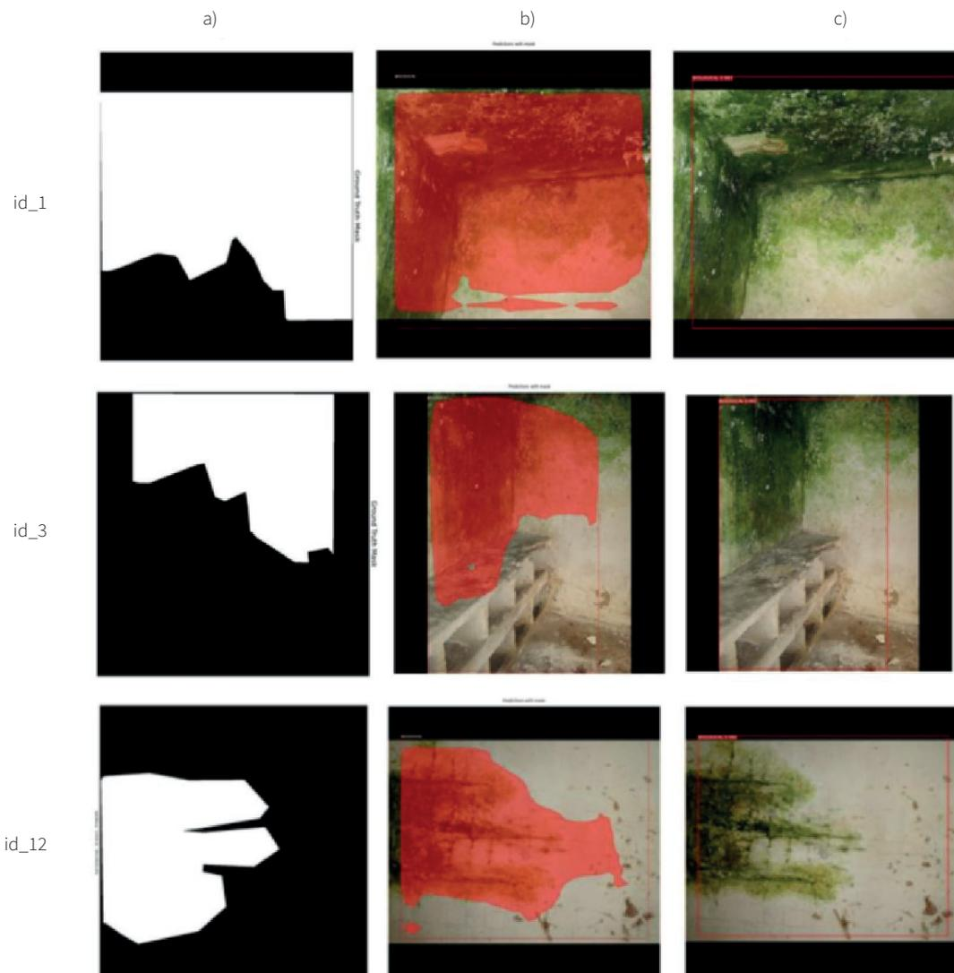
**Figure 3** | a) ground truth mask (transposed image); b) segmentation mask; c) bounding box, for biological colonization
