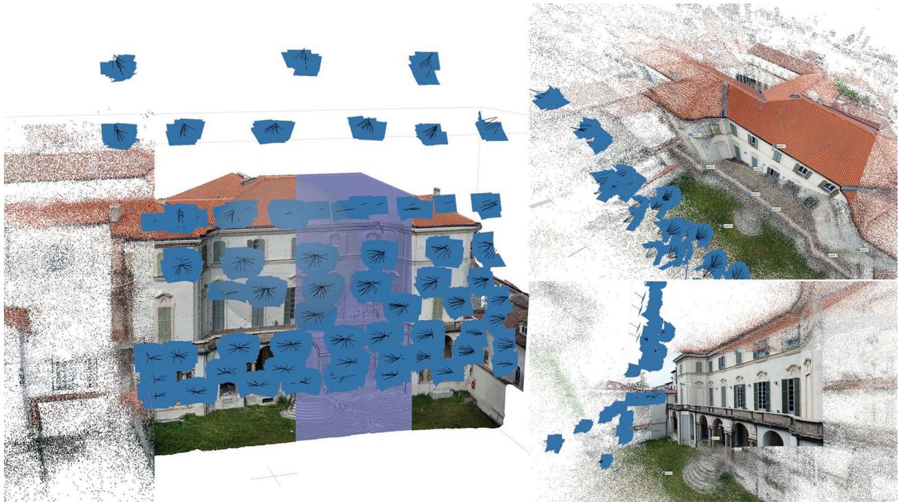
**Figure 8** | Close-range photogrammetry of the facade on the Palace garden performed with DJI Mavic mini. Left: the evolution of processes from point cloud to textured model. Right: images of the sparse point cloud highlighting the location of acquired photographs and targets used for model alignment. The UAV acquisition was conducted with the support of licensed pilot R. De Marco.
