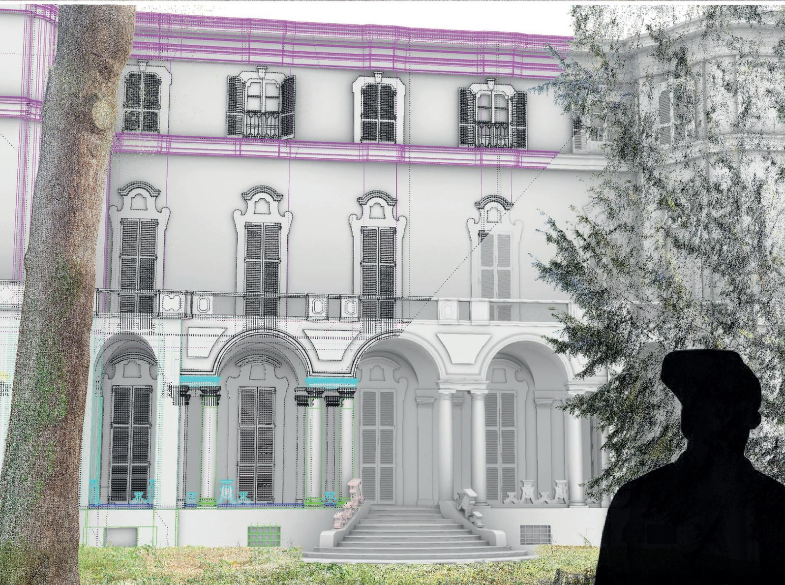
*Images extrapolated from the laser scanner RGB point cloud (top) and reality-based 3D modeling phase (bottom) of Palazzo Bellisomi Vistarino, Pavia*
