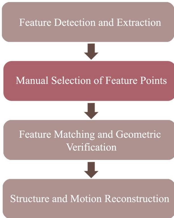
Figure 3 | Flowchart of the customised SfM pipeline applied on historical images in which a step (in red) of Manual selection of Feature Points was added to the standard SfM pipeline in COLMAP.
