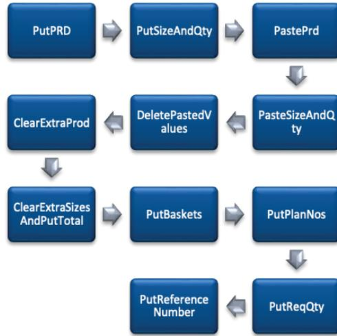
Figure 9: Macros and their execution sequence when the command button (initialize is clicked).
