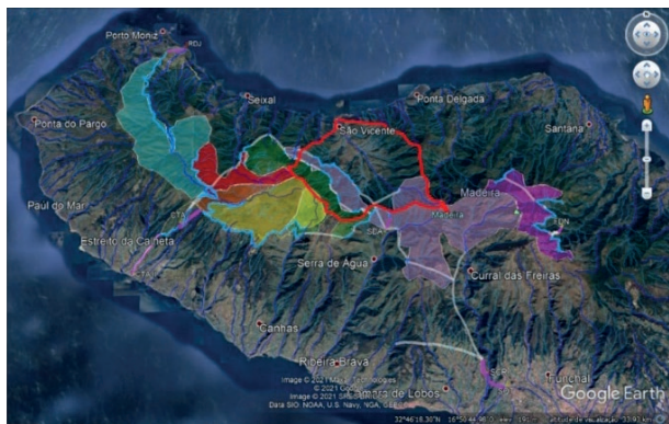
Figure 7: Catchment areas (coloured spots) and respective hydroelectric power plants (pink lines).
