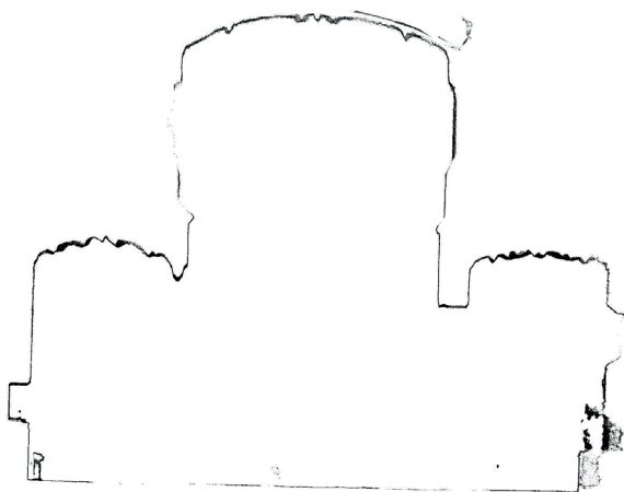
Fig 15. Partial point cloud slice integrating nave and space under the roof in a cross-sectional view of the ensemble. Source: Own elaboration with Manuel Viola in 2022 based on Ortiz & Cabecera 2022.
