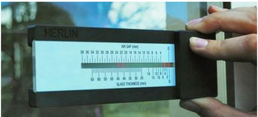
Figure 6. Glass thickness measure using Bohle, Merlin Laser device
