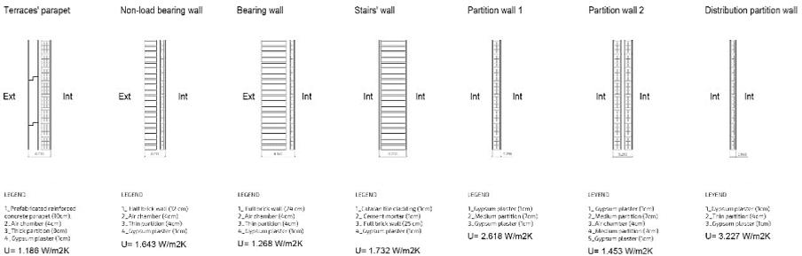
Figure 8. Thermal transmittance values obtained by the simulation software for the existing constructive system
