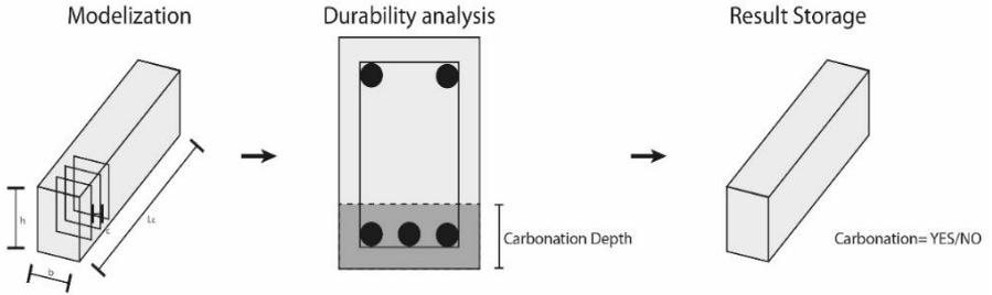
Figure 3. Steps for the durability analysis
