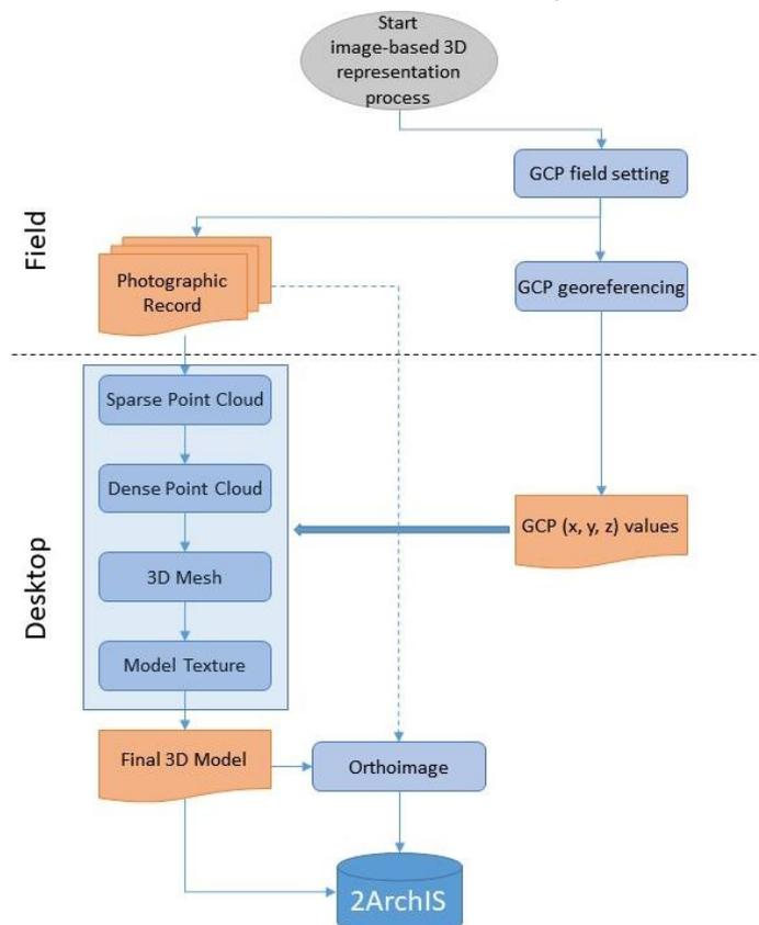
Figure 2: Simplified workflow of the 3D reconstruction process
