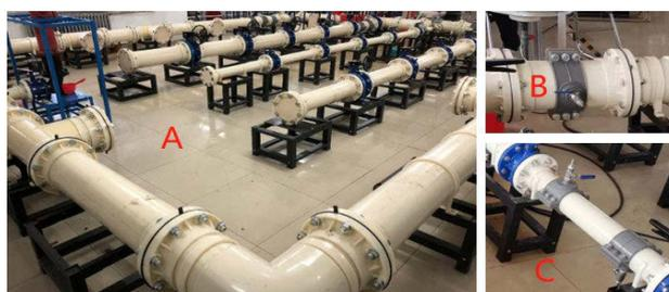
Figure 1. Full-scale water distribution system experimental device
