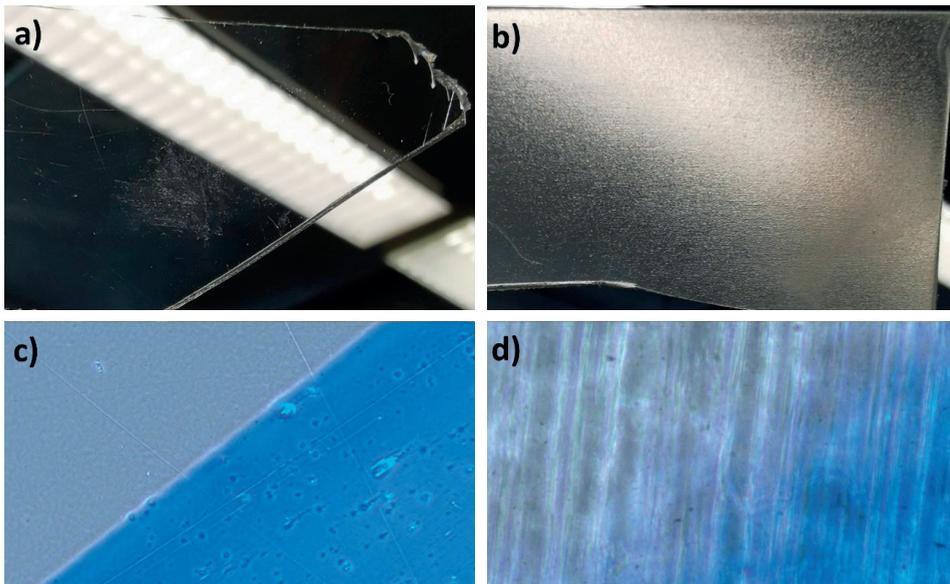
**Figure 4.** Visual comparison of transparency of new cell culture flask (a) and recycled material (b) and microscopic inspection of the surfaces (c: new PS; d: recycled PS). To adjust sharpness on the microscope, a blue line was drawn on the materials.
