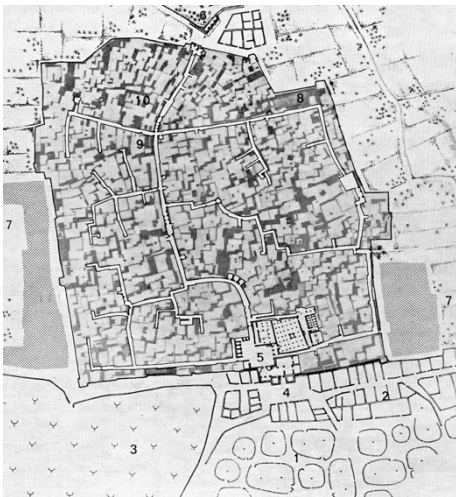
Fig. 5- Surveyed plan of the Goulmima Ksar in the 1960s. Legend: 1: Threshing areas, 2: External stables, 3: Cemetery, 4: Entrance and guard room, 5: Main square, 6: Washhouse-drinking trough, 7: Extension, 8: Internal stables, 9: Former east gate, 10: Jewish quarter (Mellah). Source: A+U n°5.
