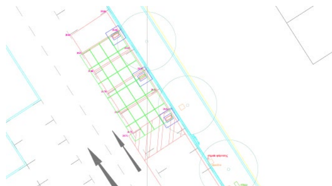
Fig. 3 – Placement of PV modules at the pilot site
