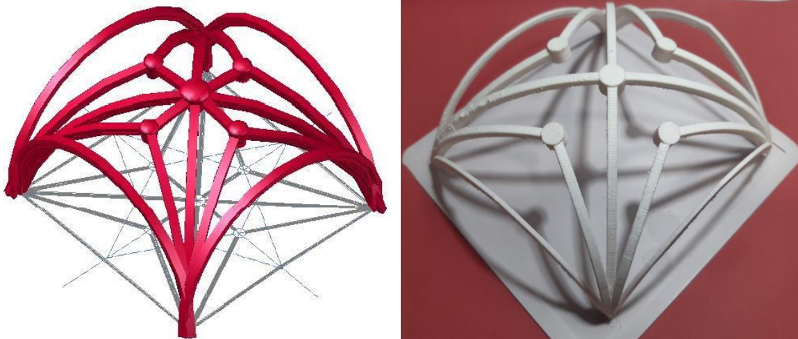
Figure 3. Model of a vault and 3D printed model. Source: Mañez, MJ. & Garfella, J. (2024)
