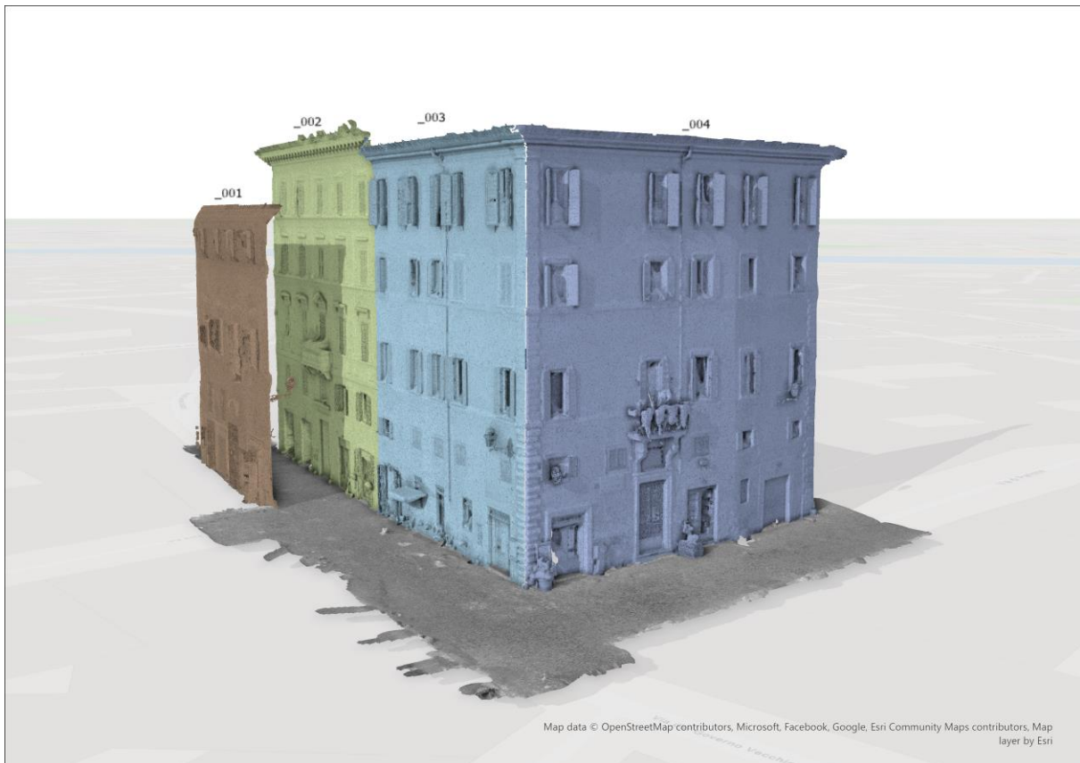
Figure 8. The collaborative model in ArcGIS with the segmented facades. Source: Author's elaboration.
