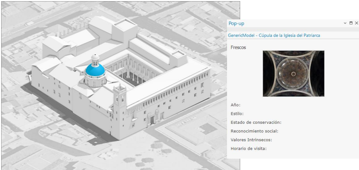
Figure 3. Example of an HBIM model highlighting a dome as a heritage element along with its data sheet in ArcGIS. LOD3, LoD500. Source: Own elaboration.
