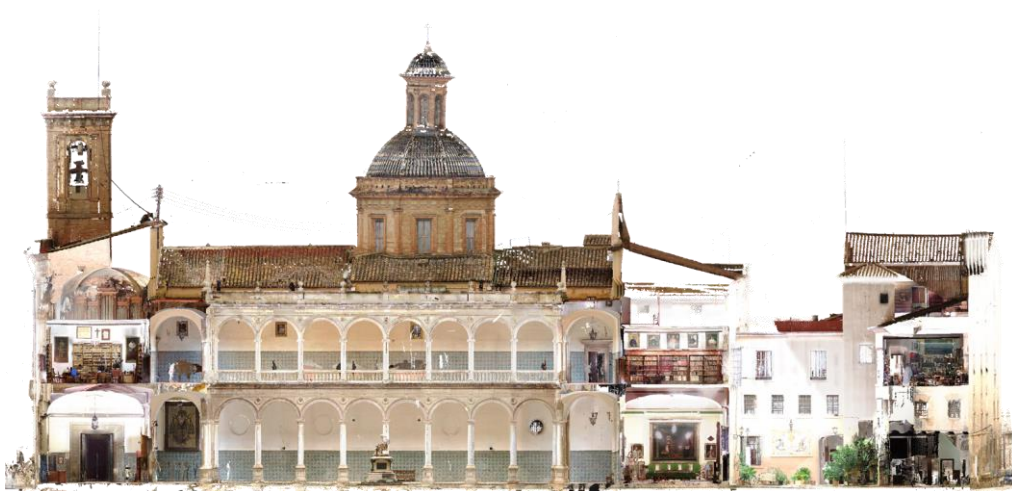
Figure 7. Orthophoto of El Patriarca's longitudinal section through the cloister extracted from the point cloud. Source: Rolim, R.
