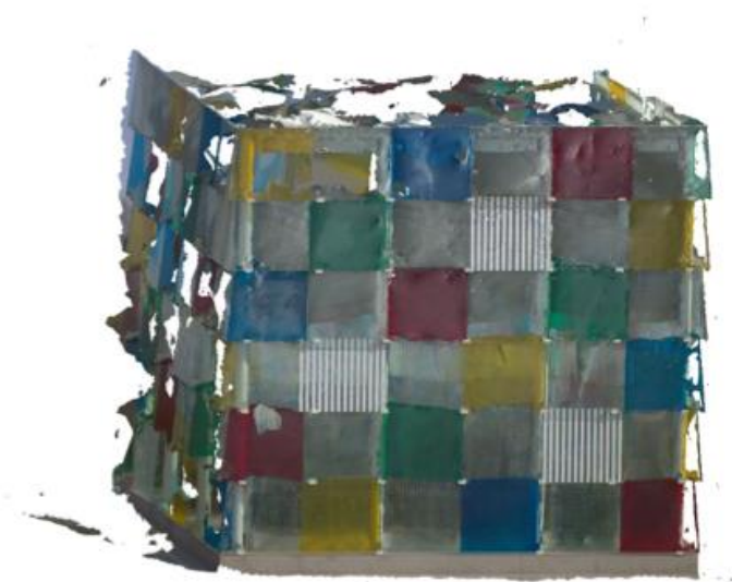
Figure 8. 3D model generated from dense point cloud. Author of the image: Deborah Fernandez León, 2024.
