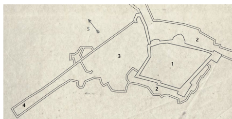
Fig. 1- The layout of St. Michael's Fortress in Šibenik; 1 - castle; 2 - faussebrayes ; 3 - place-of-arms; 4 - strada di soccorso (Pavić, 2021).
