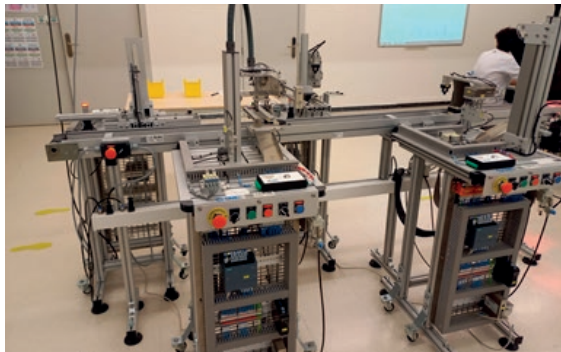
Figure 5. Representation of the FAS-200 Assembly line.
