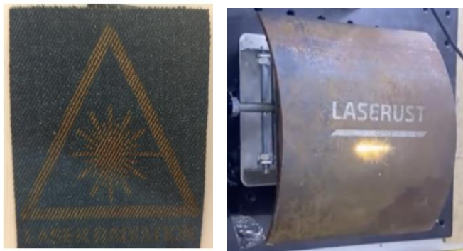
Figure 2. Left. LaserJeans (2018-2019) example of laser drawing on denim fabric. Right. Laserrust (2021-22) example of laser rust removal showing their logo.
