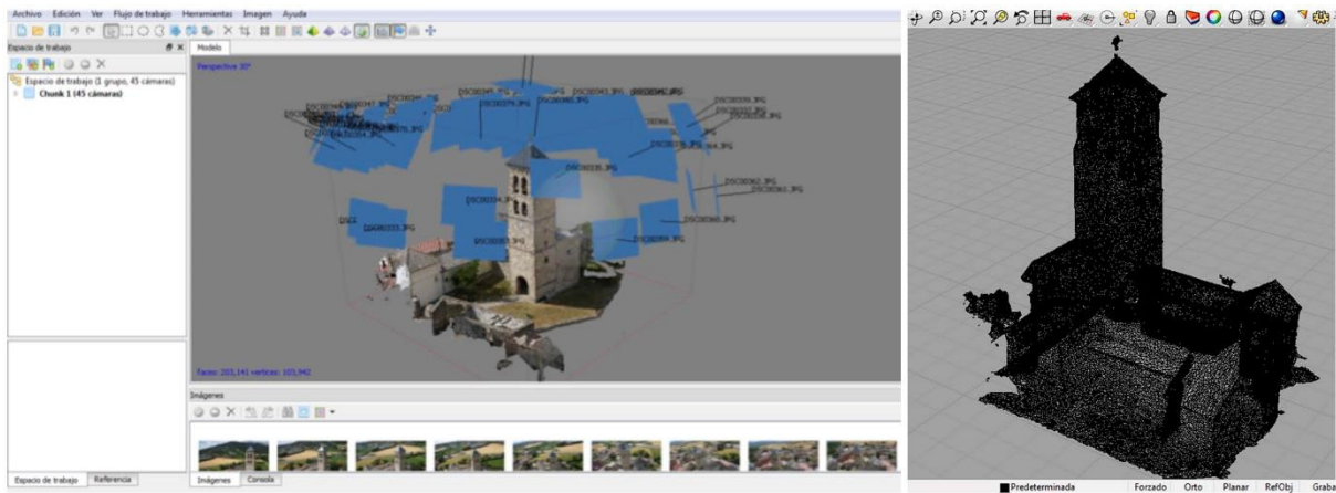
Figure 10. Virtual reconstruction process of the model with photogrammetry. Source: Muñoz, C.; Piedrafita, J. (2015)
