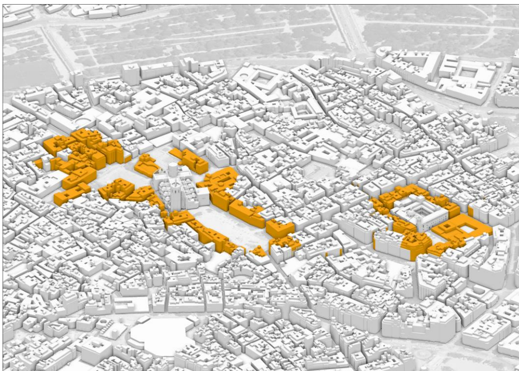
Figure 4. Example of OLOD1 building context in ArcGIS highlighting the protection areas of two heritage buildings. Source: Own elaboration.
