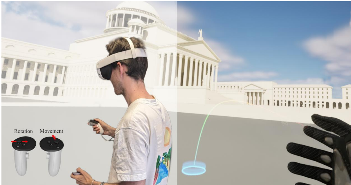
Figure 5. Navigation of the virtual environment using the teleporter with the joystick. Source: Vanni, E.
