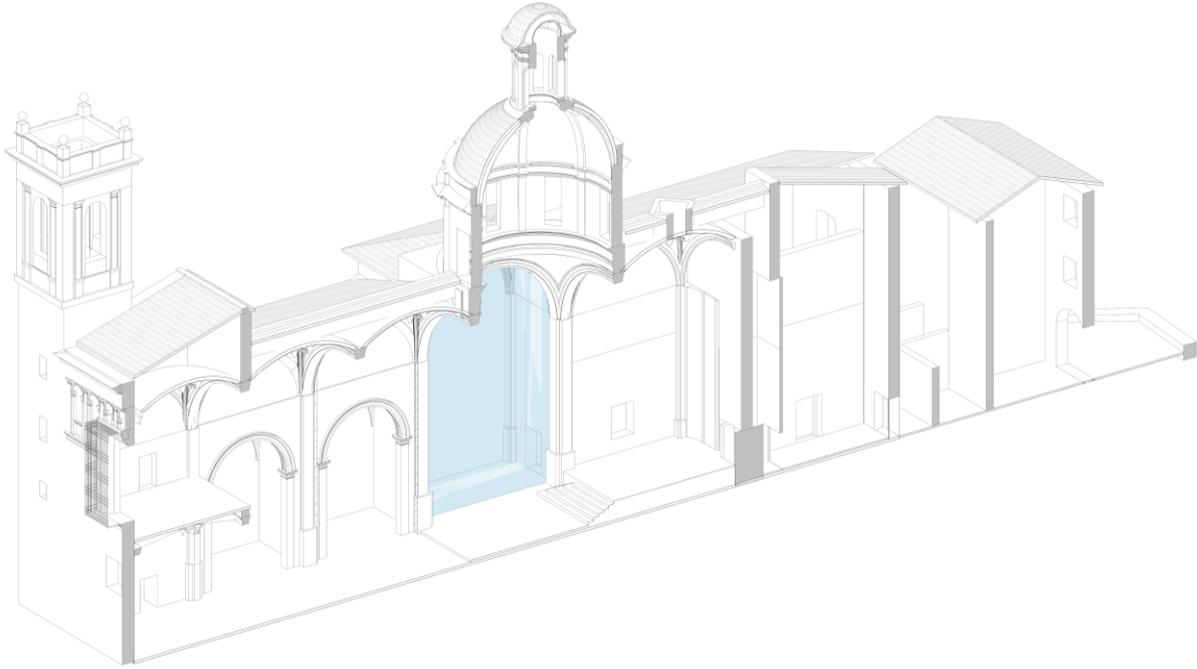
**Figure 9.** 3D volume visualised inside a 3D section of the Colegio del Patriarca church. Source: Own elaboration (2024).
