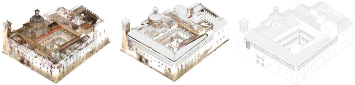
**Figure 3.** Point cloud of Colegio del Patriarca; Point cloud superimposed on the 3D model; 3D model of Colegio del Patriarca under development. Source: Own elaboration from the point cloud taken in 2023 by PhD Junshan Liu.
