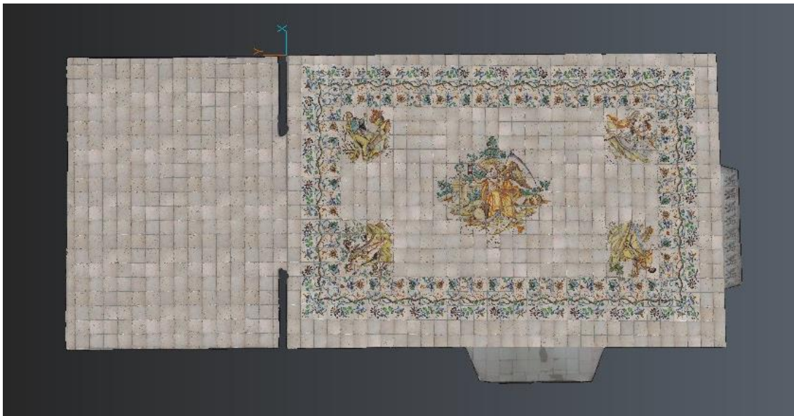
Figure 13. Pavement texture adjusted to the mesh. Floor view.
