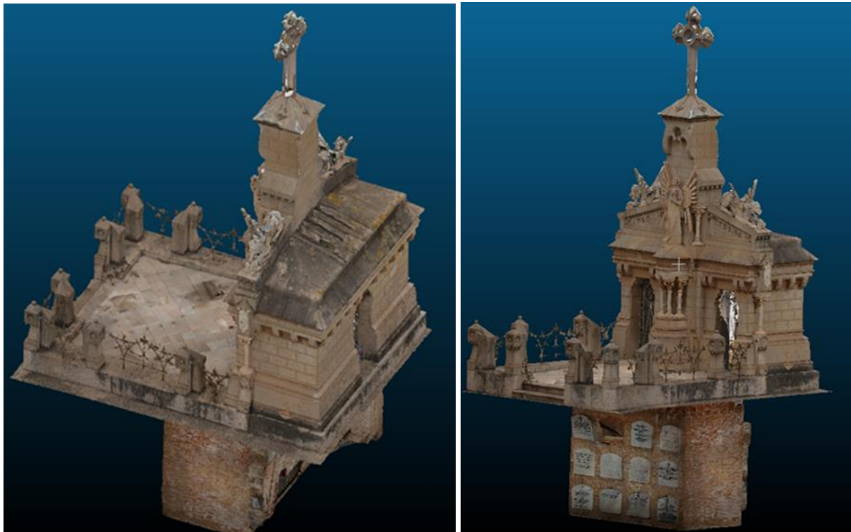
Figure 11. Joint mapped and textured triangle mesh of the Cortina family Pantheon
