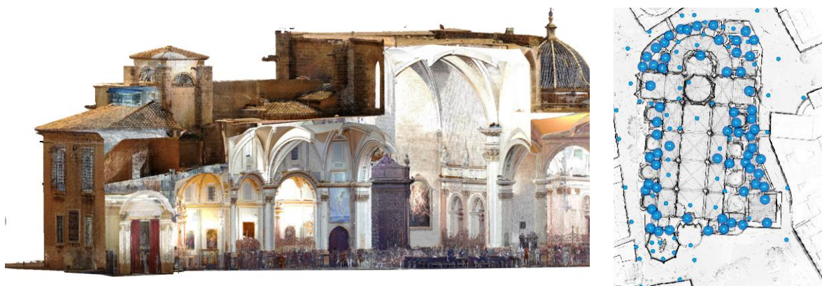
Figure 4. Left. Point Cloud image of the Cathedral of Valencia Right. Scan positions inside the Cathedral and its surroundings. Source: Escudero, P.A.
