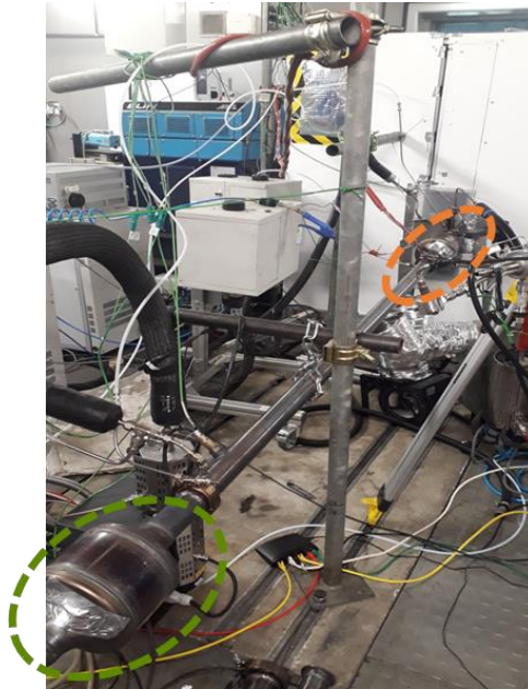
Fig. 2. GPF setup for engine bench tests, Close Coupled (CC) GPF in orange, Tailpipe (TP) GPF in green
