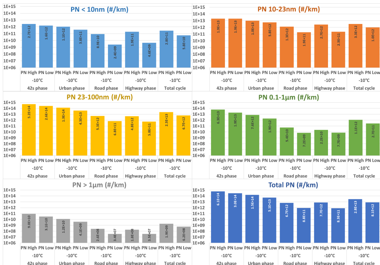
Fig. 20. Averaged engine-out PN10 spectrum with Fuel PN High and Low at -10°C
