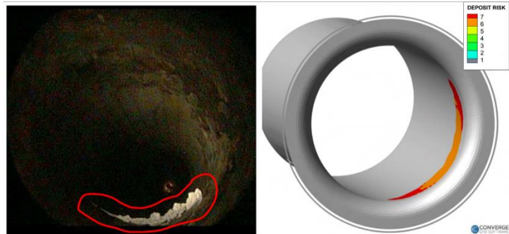
Fig. 17. OP4 deposit formation: exp (left) and sim (right)
